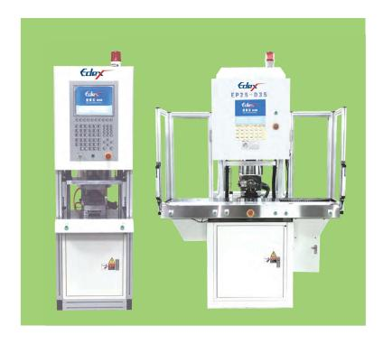
Servo Motor for Packaging Injection and Mold Clamping / Opening Pneumatic Pressure for Injection Unit and Ejector
